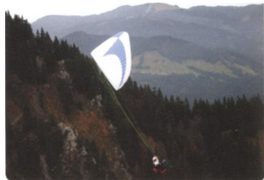
Picture 6.16 Sometimes the wing may be pitched back quite far when it meets the rising air inside the thermal. In extreme cases paragliders may enter a deep-, or even a full stall, due to this pitching motion. If this happens, first solve the problem, and then consider if this thermal is ok for you.
