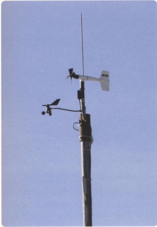
Picture 7.26 Dedicated anemometers are even more sensitive than wind socks. Furthermore they are generally placed on higher stakes and thus give a more correct reading - but they are small and can only be seen from close by. Wind streamers also need less wind than true windsocks.
