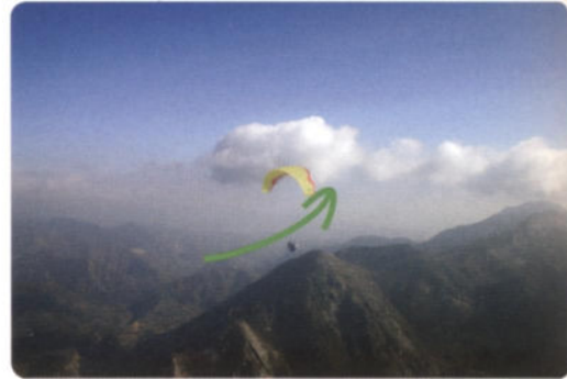
Picture 4.56 How would you fly to get to this cloud? The sun is shining from the right onto the slope and the upper wind is also blowing from the right. Both indicate that the cloud should be approached at its right end (arrow).
