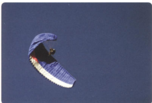
Picture 10.9 Small collapse caused by a wing-over gone wrong. Docile wings forgive most of our mistakes while Open Class wings may show hefty reactions to such mishaps.
