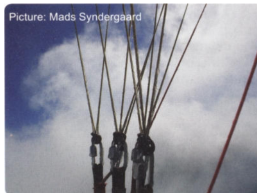
Picture 4.15b After 10 minutes inside the cloud the condensation starts running down the lines. The brake line becomes a small inverted fountain, the water soaks first the gloves, then sleeves and back of the pilot. If it is cold the water freezes and thick layers of ice may form, see picture above.
