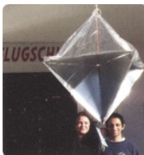
Picture 9.1 This radiosonde was found in the Isartal. The instruments are attached to the lower end and transmit the soundings back down to earth via radio.
