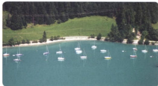
Picture 7.21 The anchor is always fastened at the bow, and the mast is closer to the bow than to the stern. Since the boat will always align itself with the wind, boats at sway are excellent wind direction markers. In this photo the wind is quite weak, or the water would be more disturbed.
