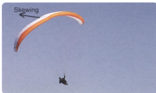
Picture 6.1 Weight shift causes the wing to distort along the centre cell. This in turn causes a skewing of the total lift vector over to the weight shifted side, and it is this skewing that makes the wing turn.
