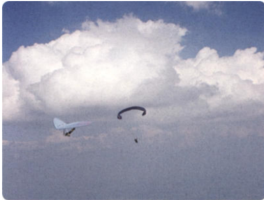
Picture 4.28 In order to escape from clouds sucking too much, the paraglider pilot pulls in his ears and pushes the speed bar, and the hang glider pulls in and dives out.
