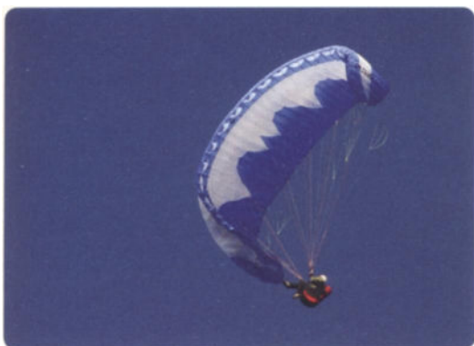
Picture 10.6 The glider suffered an asymmetrical collapse, immediately followed by a counter-collapse on the opposite side. Both collapses would have been avoidable for the skilled pilot, but the glider is a forgiving model and has hardly changed its heading.
