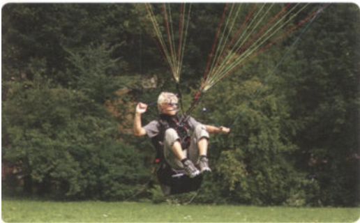
Pictures 10.23 Playing with our favourite toy. If you're not wearing your harness, steering with the A's and D's is the easiest way. With the harness the D-risers are still useful for steering but remember to wear gloves when you grab paraglider lines - they make painful burns. If the wind gets stronger you should ALWAYS wear a helmet.
