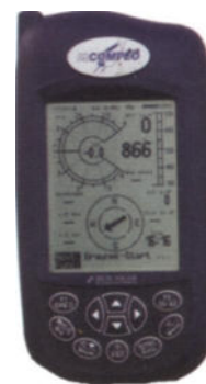
Picture 6.7 A high-end modern vario with TEC options built in.
