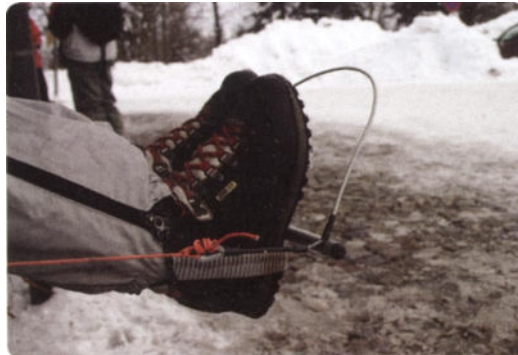
Picture 0.9 Standard speed bar with an angled 1st step to ease the stepping into. The wire loop is used with one foot to get in, then both feet move to the actual rod and slowly accelerate to the desired speed.
