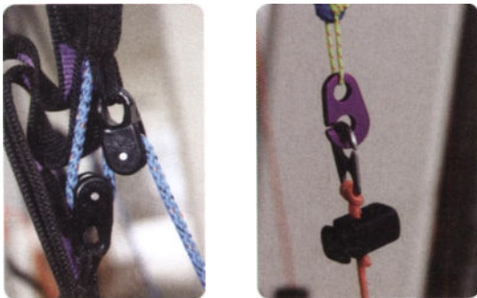
Picture 0.7 Pulley-to-pulley at top speed. In this picture approximately one more centimetre may be pushed.
