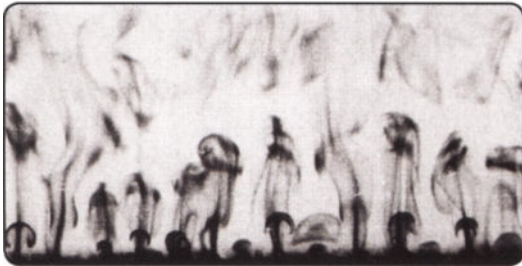
Illustration 1.33 These pictures were produced by the University of Stanford in California. They show oil being heated by a hot plate, with "thermals" rising from the bottom. The photo above shows the ideal situation, with beautifully formed and regular shapes. The lower picture shows the same situation but now the hot plate has been turned up too high; the "thermals" rise too fast and in a chaotic manner. This compares well to lee thermals or to airmasses where the temperature gradient is too high, see also page 219: A temperature gradient of minus 0.9 - 1.0 deg/100m.
