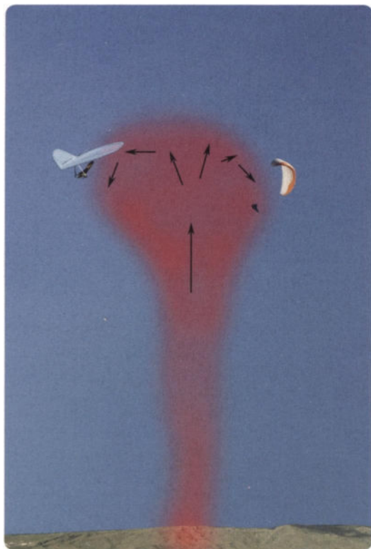
Illustration 3.1 Strong thermals cause strong turbulence. If the pilot falls out of the side of the thermal the wing may dive very aggressively. It is not dissimilar to a surfer falling off the lip of a wave.
